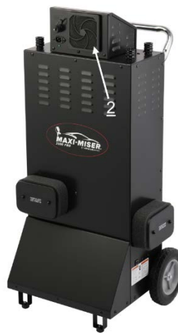
Fan filter – control panel
